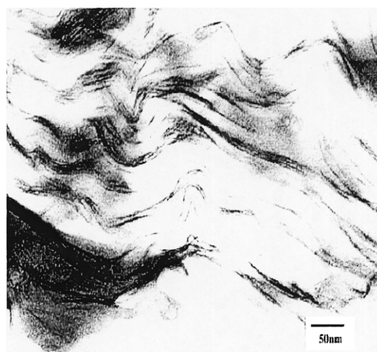
Fig. 4. TEM of a 1% PAI nanocomposite showing face–face coagulation, edge–edge flocculated tactoids in an exfoliated nanocomposite.
